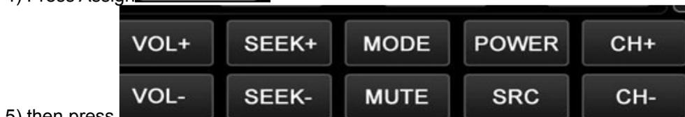
5) then press according to your record just now ( for example , just now you press the first button on the steering wheel , the first button is Vol+ ,
